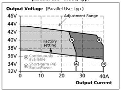
Fig. 6-4 Dynamic overcurrent capability, typ.
