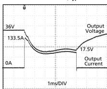
133.5A Peak load (resistive) for 5ms Output voltage dips from 36V to 17.5V.
