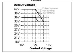
Fig. 10-2 Applying the control voltage
