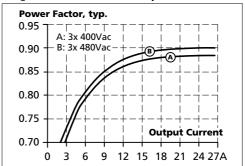
Dec. 2016 / Rev. 1.3 DS-QT40.361-EN All parameters are specified at 36V, 26.7A, 3x400Vac, 25°C ambient and after a 5 minutes run-in time unless otherwise noted.
