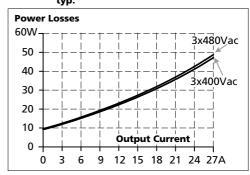
Fig. 11-4 Losses vs. input voltage at 36V, 26.7A, typ.
