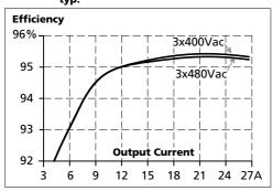
Fig. 11-3 **Efficiency vs. input voltage at 36V, 26.7A, typ.**
