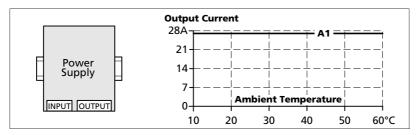
Fig. 24-11 Mounting Orientation B (Upside down)
