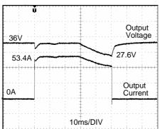
53.4A Peak load (resistive) for 50ms Output voltage dips from 36V to 27.6V.
