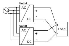
If more than three units are connected in parallel, a fuse or circuit breaker with a rating of 32A or 40A is required on each output. Alternatively, a diode or redundancy module can also be utilized.
