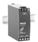
The YR40.482 is equipped with two input channels (20A each), which are individually decoupled by utilizing mosfet technology. The output current can go as high as 40A.
